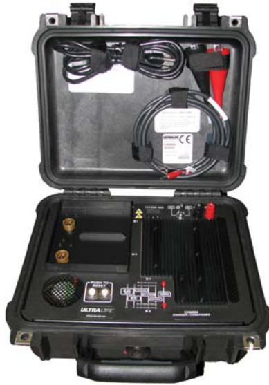
Figure 1: CH0004 Charger (Front View)
